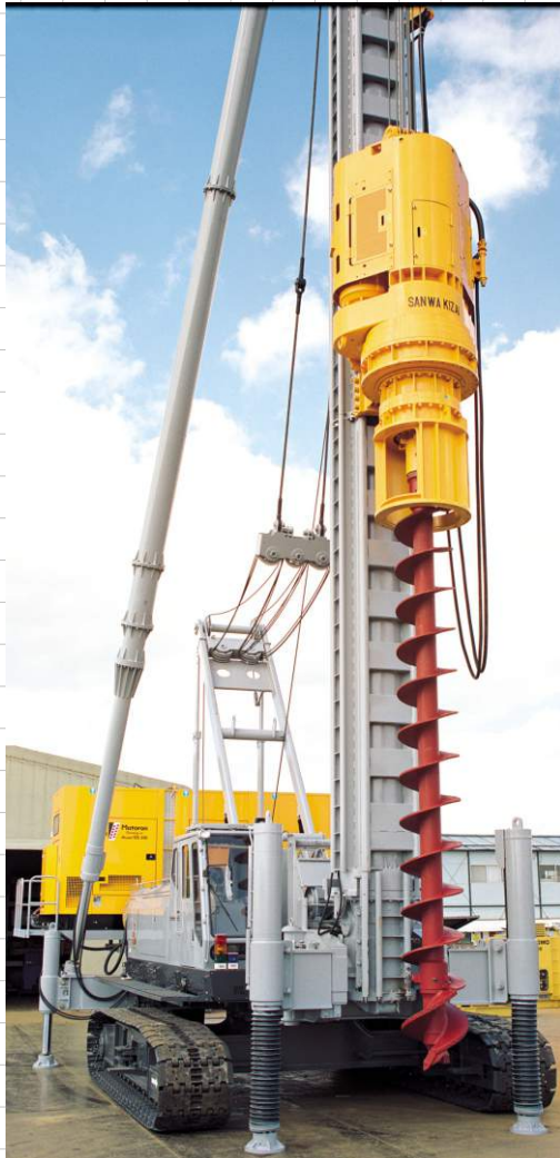
Sanwa Kizai SMD-150HP Doughnut Auger Boring Machine
